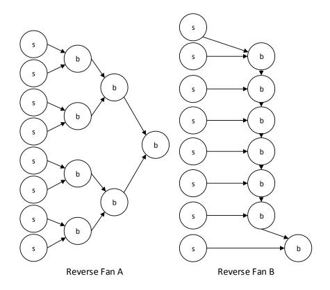
Figure 17: The dependency graph of the reverse fan benchmarks.
